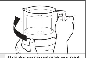
Hold the base steady with one hand, and use the other hand to rotate the work bowl clockwise to unlock and lift it off of the base.
