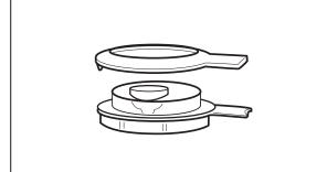
**OPTIONAL:** The lid ring can be removed for more detailed cleaning if necessary.
