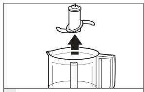
Pull the blade straight up to unlock 2 and remove it from the work bowl.
