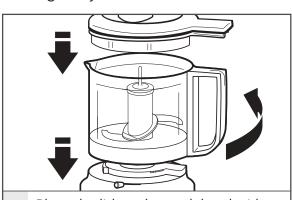
Place the lid on the work bowl with the lid handle facing front. Rotate the lid handle to the right. Rotate the lid counterclockwise to lock into place.
