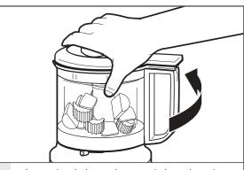
Place the lid on the work bowl with the lid handle facing front. Rotate the lid handle to the right. The lid will click when locked into place. Rotate the lid counterclockwise to lock into place.
