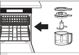
The work bowl, lid, lid ring, and blade can be washed in the top dishwasher 2 rack or, wash all parts in hot, soapy water. Rinse and dry.
