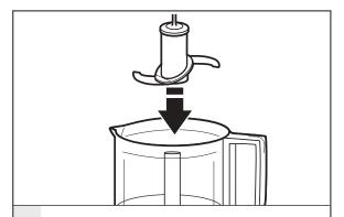
Fit the blade over the shaft in the centre of the work bowl, rotate and press down until it locks into position.
