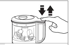
For a coarse chop, use a pulsing motion to rapidly press and release the PULSE/ON button until your desired results are achieved.
