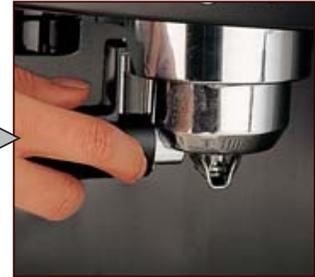
Rinse filters and filter-holder, and place back on the machine.
