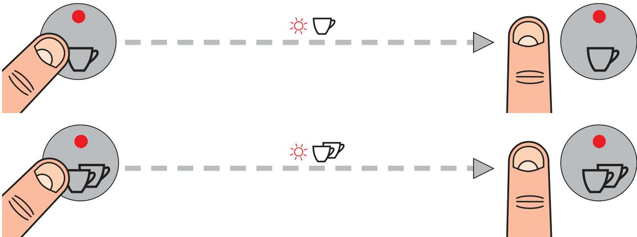
Press **and hold** button, release at desired level.
