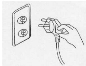
Then put the plug in a 230 volt safety-contact power outlet.
